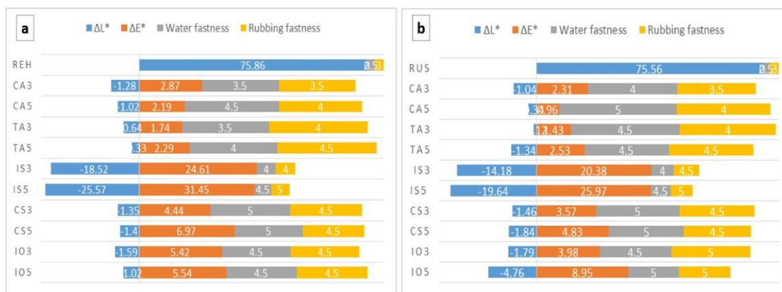
Fig. 2: Graphical representation of the difference in luminosity, colour and fastness values of samples dyed by the exhaustion method (a) and ultrasonication method (b).
